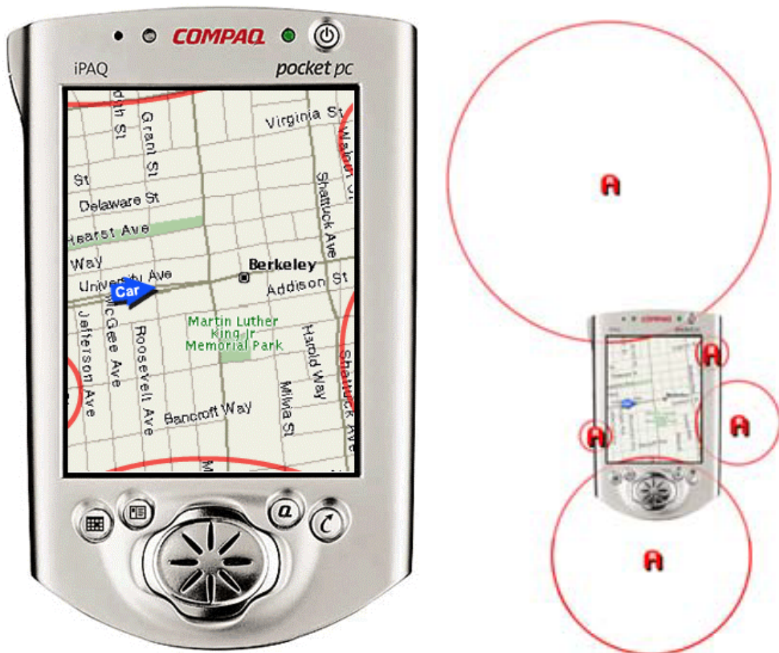
(a) Red arcs around the edges of the viewport indicate locations of off-screen elements.
